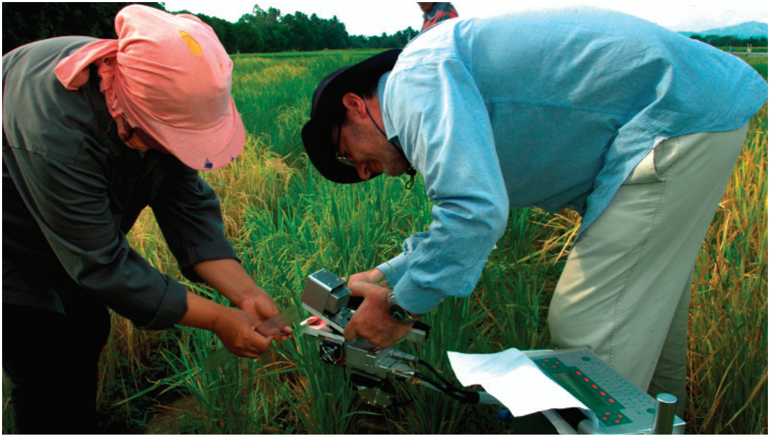
Mauro Centritto (right) from Consiglio Nazionale delle Ricerche, Rome, Italy, helps an IRRI technician measure photosynthesis using a Li-Cor LI-6400-40 Leaf Chamber Fluorometer.
